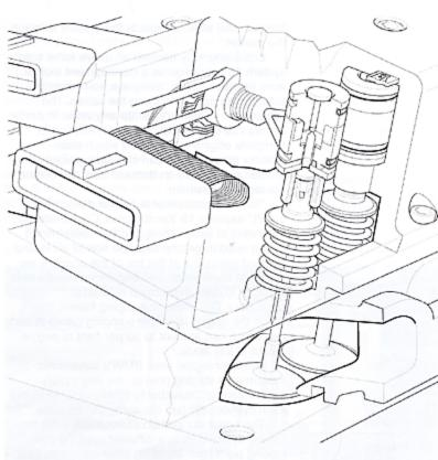
Lotus AVT: flexible control over valve lift and timing.
