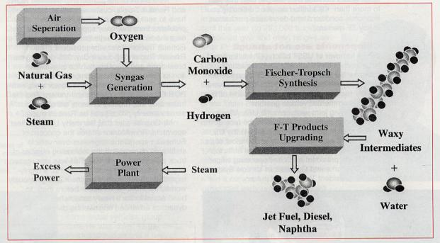
Fischer-Tropsch catalytic synthesis: at the heart of the multi-stage gas-to-liquid production process. Source: Mitretek Systems.
