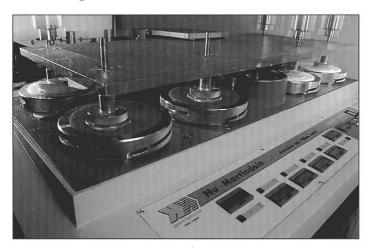
The apparatus records the number of cycles - or rubs - to which the fabric has been exposed until a physically significant end point is reached. The end point is when three threads on the fabric have worn to the extent of actually breaking and the abrasion value is the number of cycles completed at the time of breaking. The fabric is abraded at a pressure of 800g/12 Kilo Pascals and abradants are changed every 50,000 cycles.
